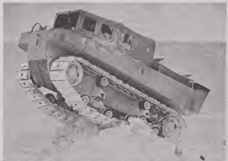
FIGURE 33. Pilot model of T-15 Weasel equipped with production grouser and climbing a snow pinnacle.
